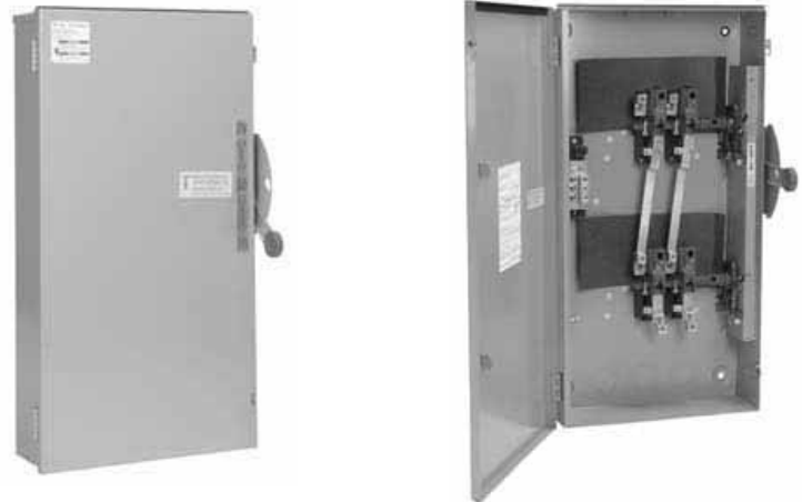
DT224URK-NPS General-Duty, Non-Fusible Double Throw Emergency Power Safety Switch, 200 Amperes, 120/240 Volts
